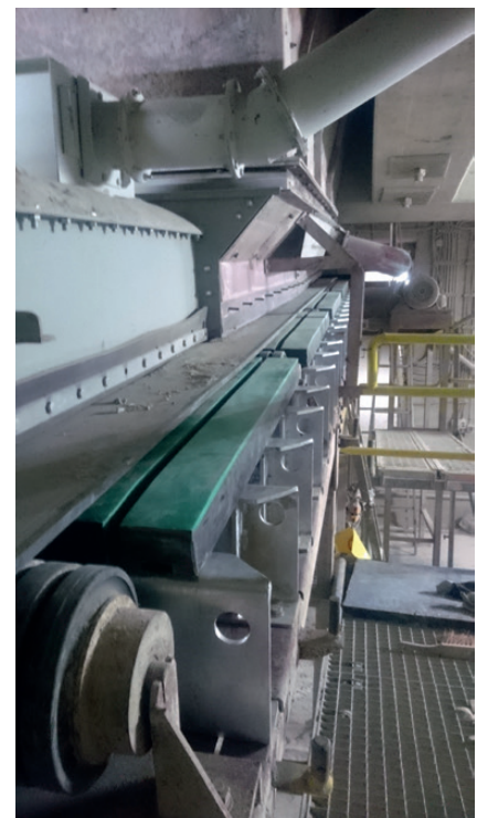
Impact table with damping element
