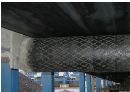
Correction roll with rubber rhomb covering
