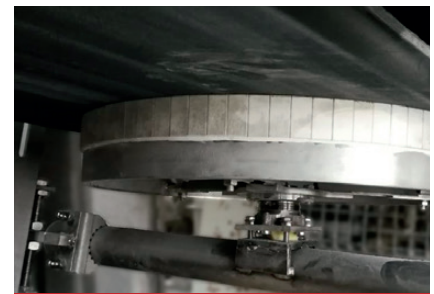
ROTA with ceramic scraping element
