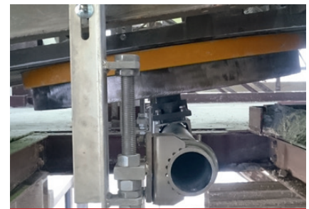
ROTA with polyurethane scraping element
